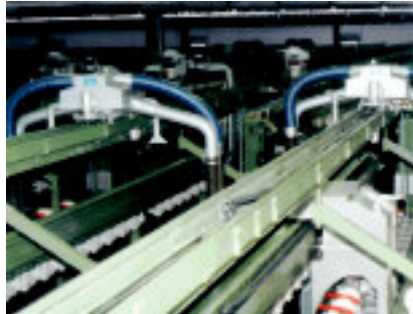
Long travel applications of up to 40 m are possible. Here: Series 10 in a textile machine
