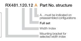
Strain relief e.g. clamps, tiewrap plates, nuggets and plug-in clips are available from stock. The complete chainfix range with order options ▶ from page 656
