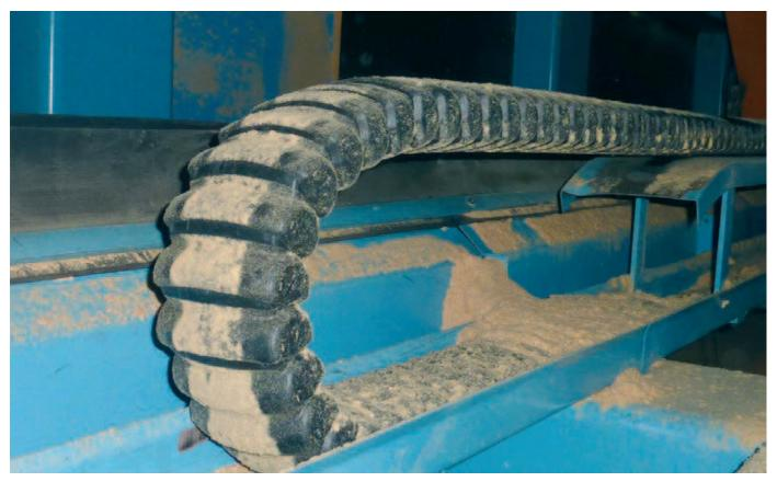
With the extreme tight igus® RX e-tube and the harnessed chainflex®-cables, the lifetime of this woodworking machine could be considerably increased. Because of dust and dirt, most after one month previously installed cables failed
